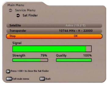
If you do not have a meter for adjusting your reflector, you can use the sat finder as an alignment aid. You can select the different lines using the volume buttons. Make changes in the lines using the buttons (e. g. transponder). Once you have a good reception signal (see example above), press the V button in the "Exit" line.
